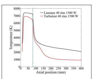
**Fig. 1**. Comparison of temperature profile along the symmetry axis, for laminar (black) and turbulent (SST; red) flows, at 1 atm. The start of the afterglow is indicated by the vertical dashed line.
